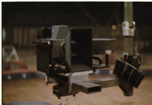
In order to achieve the requisite vertical format to fit space allotted in the Circus Museum, it was necessary to mount a Todd-AO 70mm camera on its side. At first the magazine jammed in this position, but Director of Photography Jack Priestley had experienced the same problem when shooting the old three-strip Cinerama and solved it in the same way—by installing special flanges inside the magazines.
