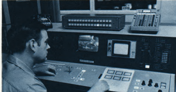
(LEFT) Myriad special effects are available if the film/tape post-production is routed through a control room switcher such as the one shown. Film director Phil Squyres and Stanford Agency producer Ken Heckman plan electronic matting for commercial. (CENTER) Assistant videotape supervisor Lloyd Rodgers programs HS-200 computerized video disc recorder for special effects. (RIGHT) Richard Carlson fills an order from advertising agency producer Mike Walman for both two-inch and one-half-inch videotape copies of commercials originally filmed in 16mm.
