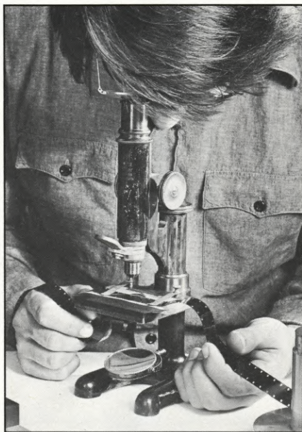
Duncan staffer in Chicago uses a microscope to check film focus on exposed and developed negative, run through a newly arrived camera.
