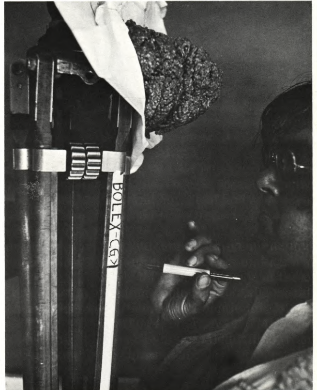
(LEFT) With utmost precision, Haddley weighs hamburger to be used as substitute weight for determining center of gravity (CG) of camera, when mounted on tripod. Hamburger proved to be ideal material for this purpose, because the weight is clearly marked on the package and it can be easily adjusted simply by adding or subtracting the appropriate amounts while watching the needle on the scale. (RIGHT) Bill Roberts points to CG (Center of Gravity) point of the tripod, with substitute weight (in hamburger) equaling the weight of the Bolex camera. The scientific method triumphs again!
