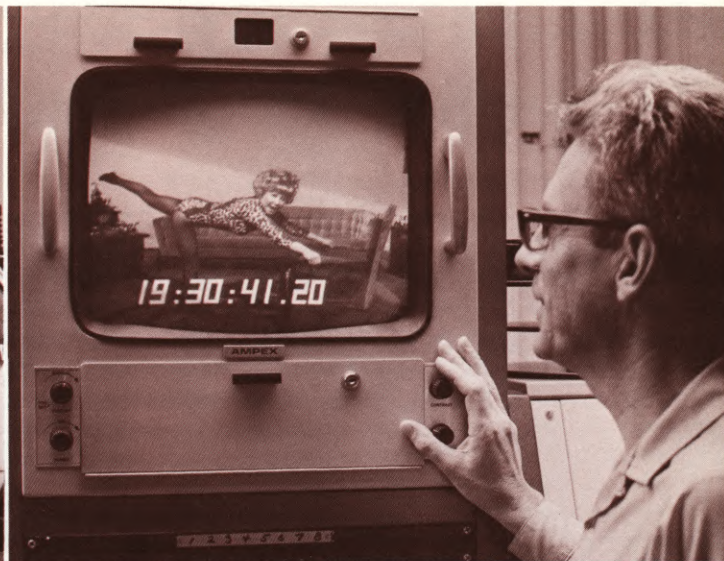
(LEFT) Film/tape production takes advantage of the economy and flexibility of 16mm location shooting. Traditional film techniques are used throughout the initial production stages. (RIGHT) Instead of the usual film workprint, a helical-scan videotape workprint is made. Each frame number appears in the screen on the tape workprint. Here videotape supervisor Bruce Harris inspects the time-code being generated during the crucial film-to-tape transfer.
