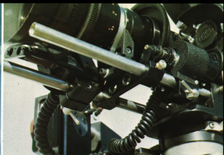
(LEFT) American Cinematographer Editor takes off in helicopter for practical test of Continental Camera Systems 35mm Mark 10 Helicopter Mount. With zoom-lensed 35mm Arriflex camera mounted, he tried all types of filming maneuvers, winding up the test by holding in closeup passengers on a fast-travelling train. (RIGHT) The mount's lens support system, showing lens and control motors securely attached to iris rods. Either motor may be easily disengaged from drive gear by simply releasing motor clamp screw and swinging unit out of the way.
