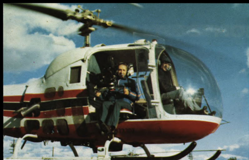
(LEFT) American Cinematographer Editor takes off in helicopter for practical test of Continental Camera Systems 35mm Mark 10 Helicopter Mount. With zoom-lensed 35mm Arriflex camera mounted, he tried all types of filming maneuvers, winding up the test by holding in closeup passengers on a fast-travelling train. (RIGHT) The mount's lens support system, showing lens and control motors securely attached to iris rods. Either motor may be easily disengaged from drive gear by simply releasing motor clamp screw and swinging unit out of the way.
