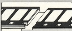
Ordinary splice leaves a bump on the film and a jump on the screen.
