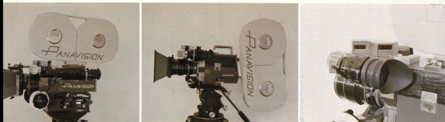
(LEFT) Panaflex camera with 1000-foot double-chamber magazine on top—extension eyepiece. (CENTER) 1000-foot double-chamber magazine mounted on the back. (RIGHT) Bright electronic digital readout for footage and tachometer. Red and green lights indicate battery condition and viewfinder displays red light if camera is not operating at exactly 24 frames per second.
