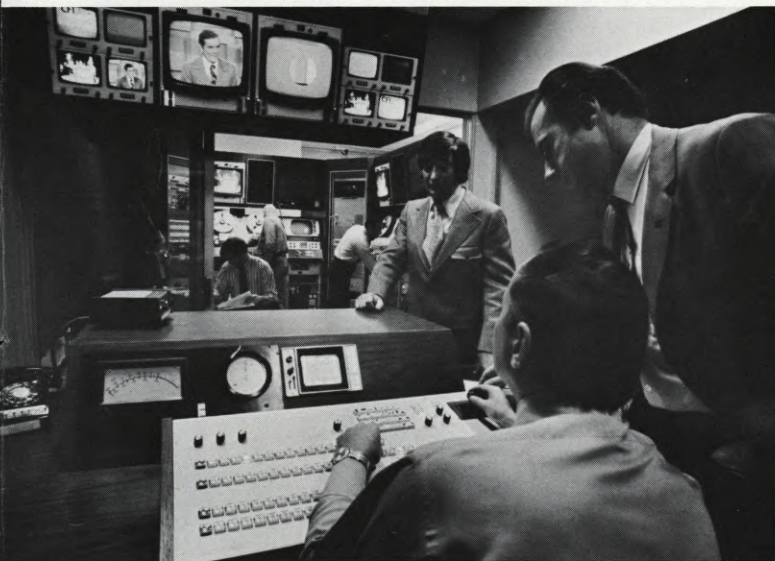
(LEFT) Master Control at CFI includes complete special effects, as well as computerized on-line editing. (RIGHT) An operator punches in a pre-program for the computerized on-line editor at CFI. At left is an Ampex HS-100 "slo-mo" recorder/reproducer. The computer will soon conform the quad tape originals automatically, including all dissolves and special effects.
