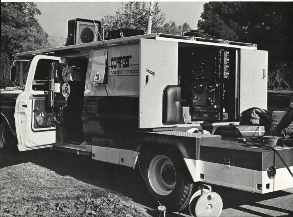
Side view of Compact Video Trucks' Mobile Unit #1. On the open door (left) can be seen the portable Ampex VR-3000 videotape recorder. In the rear is located the audio control center, complete with multi-channel audio recorder.
