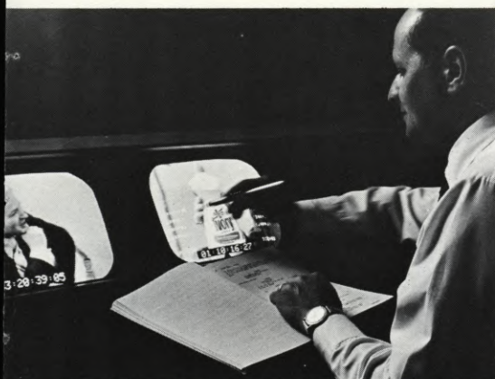
(LEFT) Editing off-line with the CMX computer. Art Schneider of Consolidated Film Industries uses the electronic light pencil, ordering the computer to make an edit. A millisecond later, the cut scene will appear on the left-hand monitor. (CENTER) The CMX off-line editor will display, upon command, a complete scene list with start and stop times for all scenes in the production. The cut show can then be recut by touching the light pencil against the appropriate scenes and edit modes. (RIGHT) The CMX "menu" consists of different commands which the computer will implement. The operator need only touch the appropriate "entree" with the light pencil.
