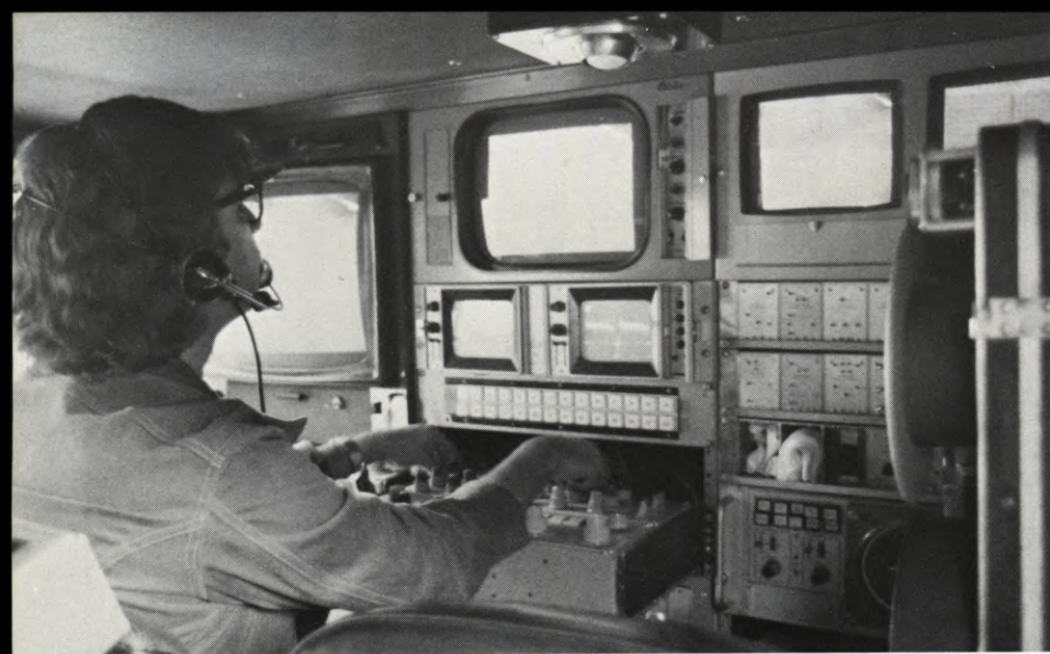
(LEFT) Inside mobile video unit's cab is the mini-control room which contains all video, switching, communications and test equipment. (RIGHT) A Golden West Broadcasters (KTLA) Telecopter hovers above the Van Norman Dam, which came near to collapsing after the 1971 San Fernando earthquake in California.
