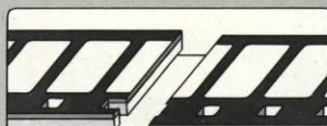
Ordinary splice leaves a bump on the film and a jump on the screen.
