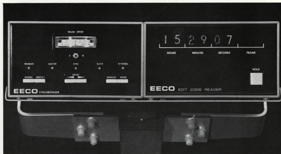
FIGURE 5 —Front control panels of BE450 Synchronizer (Left) and BE420 Edit Code Reader. These units, working in conjunction, detect the difference in the two codes during playback and generate an error-control signal to either speed-up or slow-down the capstan motor of the slave recorder until synchronization is accomplished automatically.
