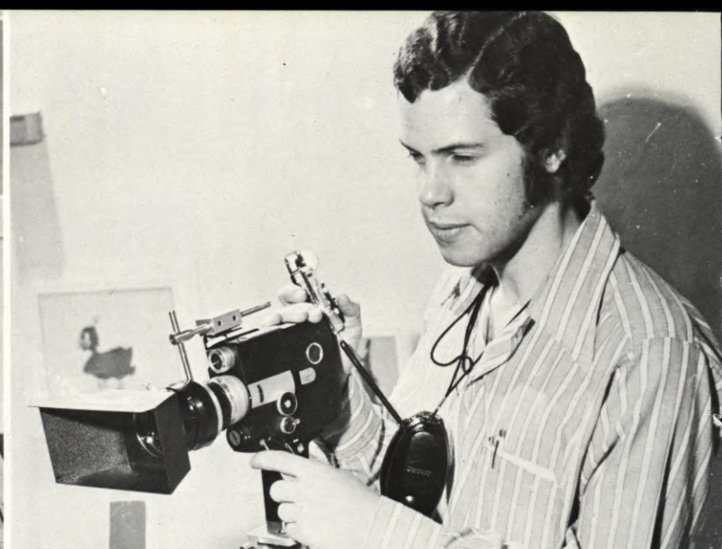
(LEFT) Eumig Mark S 712D projector, with transformer at left for stronger bulb, and anamorphic lens fitted to front of normal projector lens. (RIGHT) Cameraman Peter Benison connects Optasync to Fuji Z-2 camera prior to shooting. Note the addition of anamorphic lens and lens shade to camera.
