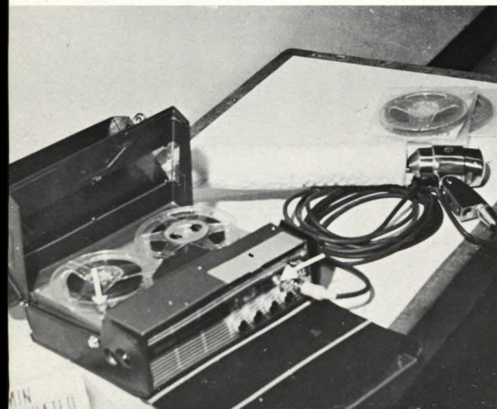
(LEFT) Uher 400 recorder converted to Optasound. Normal Optasound light-sensitive cell is usually mounted on left side of the recorder and is about 6" x 2" x 2". Arrow on left shows only evidence—light sensitive cell and light. Arrow on the right shows switch which enables camera to be started by tape recorder, or recorder to be started by camera. (RIGHT) Fuji Z-2 camera with anamorphic lens, lens shade and showing position of Optasync contacts. The camera receives pulses from sprocketed tape on recorder, so filming speed is governed by tape speed.
