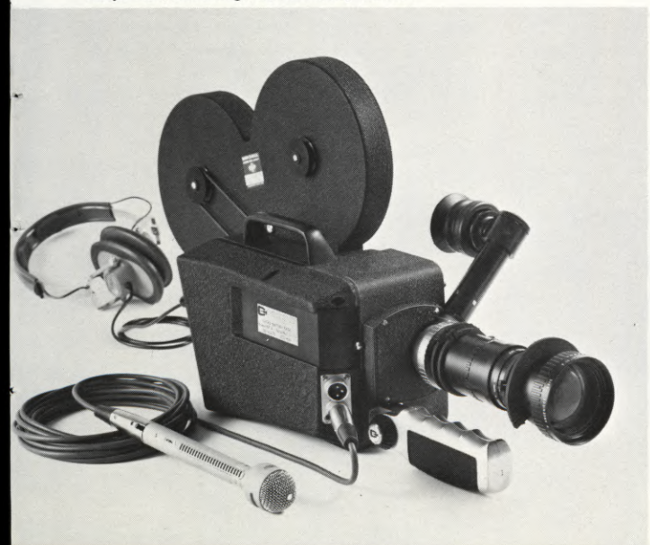
(LEFT) Front view of the CP-16A camera with Crystasound Recording System. Microphone is shown plugged into one of the two available microphone inputs located on the front of the camera. The cameraman's monitoring earphones are shown plugged into the rear panel of the built-in Crystasound System amplifier. The cameraman can monitor the live mikes while the camera is not running, and is automatically switched to the playback amplifier the moment the camera is turned on. (RIGHT) Rear view of the CP-16A camera, with Crystasound Recording System built-in amplifier, showing the auxiliary mixer.
