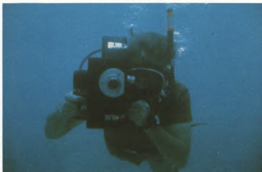
(LEFT) Joe Keyerleber sets the diaphragm by rotating the clear plexiglas "snoot" on the SeaScope camera. (CENTER) A head-on shot of Keyerleber shooting with the SeaScope. New camera is compact and easily maneuvered underwater. (RIGHT) Jack Cosgrove films hammerhead shark with Scope's original underwater camera, a Bolex H-16 in transparent plexiglas housing. After six years of service, it imploded on a shark-filming dive in 60 feet of water.
