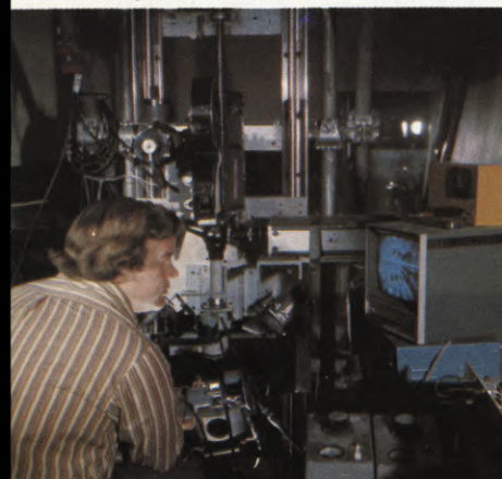
(LEFT) Director Douglas Trumbull sets up complex microscope rig to photograph what astronaut sees through his microscope. Set-up includes standard 35mm Mitchell camera, Sony TV camera, 5-to-1 Zeiss zoom microscope and special microscope stage with joystick control. (RIGHT) Originally developed for Trumbull's effects in "ANDROMEDA STRAIN", the rig has Sony video camera viewing through beam-splitter head.
