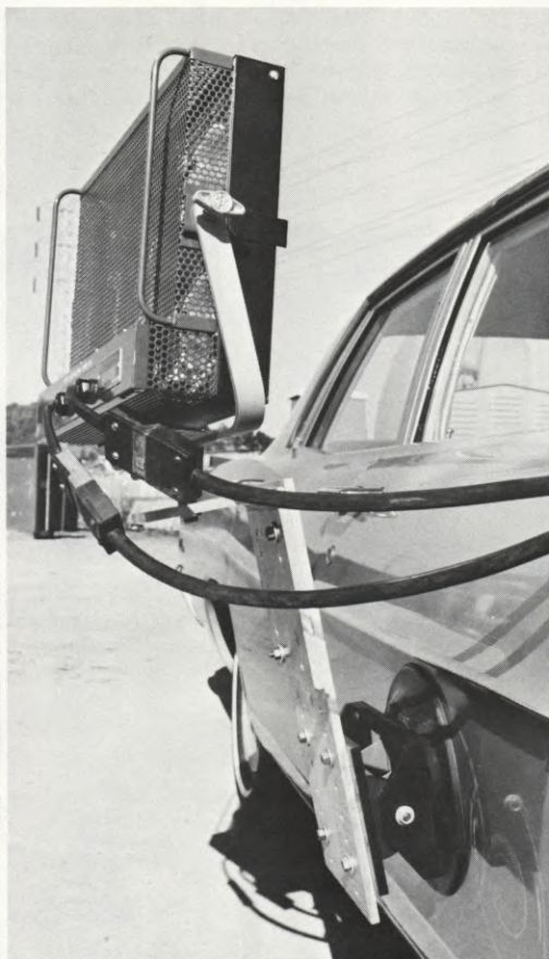
(LEFT) Designer of the Super-Grip, Ken Phelps, standing with confidence on one of his creations attached to the side of a truck. (RIGHT) A heavy five-light Molefay unit being used as a key light for a typical running shot. Note the simple extension plate used on the Super-Grip to raise the light.
