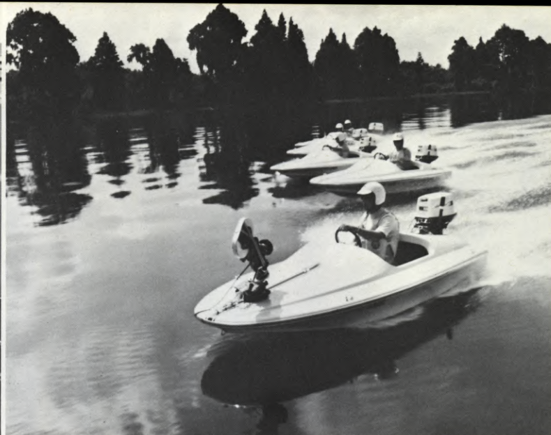
(LEFT) Three Super-Grips provide a strong support for a heavy remote pan/tilt head and 35mm Arriflex. This proved to be a rigid and reliable set-up on a coarse road at speeds in excess of 100 miles per hour. (RIGHT) A Super-Grip is used to mount a 16mm Arriflex to the bow of a speedboat for a wide-angle shot at Cypress Gardens, Florida.
