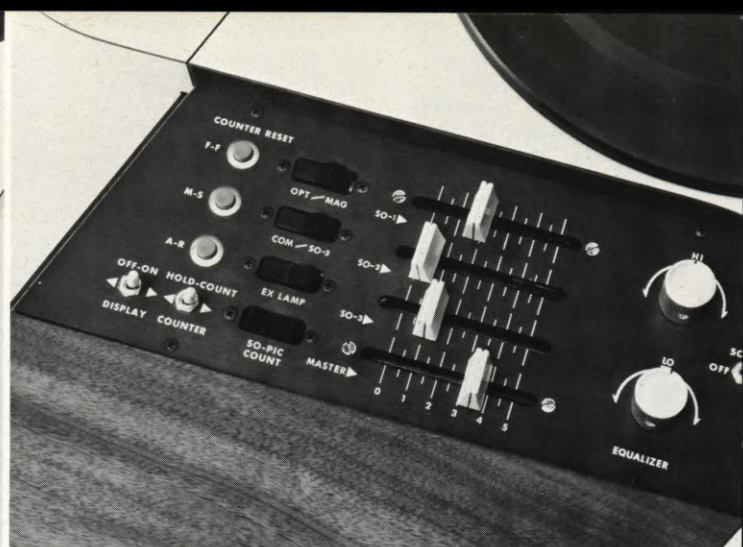
(LEFT) The control panel which is standard on all Showchron models. (RIGHT) The mixing control panel which is also standard on all Showchron models. Direct interlock drive system permits the coupling and decoupling of sound or "picture to picture" for selective composition and editing.
