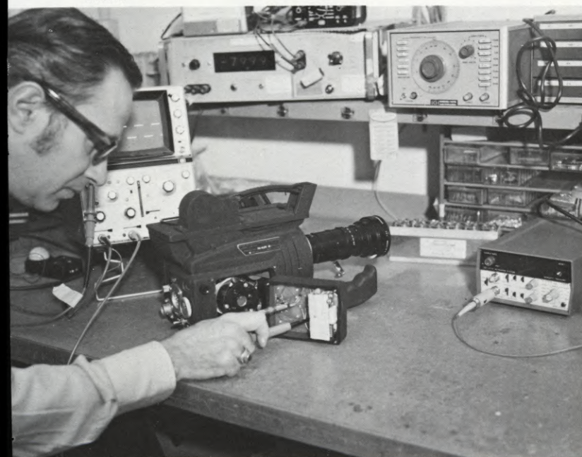
(LEFT) FIGURE 5—Each camera is given a final check for frequency and voltage after exposure to high and low temperatures. (RIGHT) FIGURE 6—The Model B-35 Power Inverter Belt for operating Auricon conversions. The belt supplies up to 35 watts of power at 120 volts AC, 50 or 60 Hz. It can be supplied with crystal-controlled output for double-system operation. A built-in charger is incorporated into the belt. Recharge time is 10 hours.
