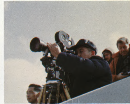
(LEFT) The fabulous camera-headed man is actually Jim Watt of NBC News. (CENTER) Watt displays his configuration of the "one-man-band" filming rig. Each cameraman had his own pet gimmicks and gadgets attached to a basic camera. The rigs averaged 40 pounds in weight, including power packs and extra magazines, carried on the shoulders and backs of the cameramen. After the third day, several were taking muscle relaxers to ease the pain. (RIGHT) Chinese cameraman filming Nixon's departure.
