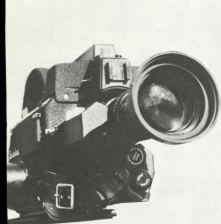
(LEFT) Front view of camera, showing power zoom and auto-exposure on-off button controls. Manual over-ride is available on both exposure and zoom controls. (RIGHT) Rear view, showing 9.6-volt rechargeable battery at rear. Battery is interchangeable in seconds.
