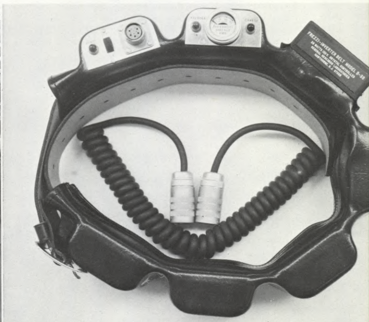
(LEFT) FIGURE 5—Each camera is given a final check for frequency and voltage after exposure to high and low temperatures. (RIGHT) FIGURE 6—The Model B-35 Power Inverter Belt for operating Auricon conversions. The belt supplies up to 35 watts of power at 120 volts AC, 50 or 60 Hz. It can be supplied with crystal-controlled output for double-system operation. A built-in charger is incorporated into the belt. Recharge time is 10 hours.
