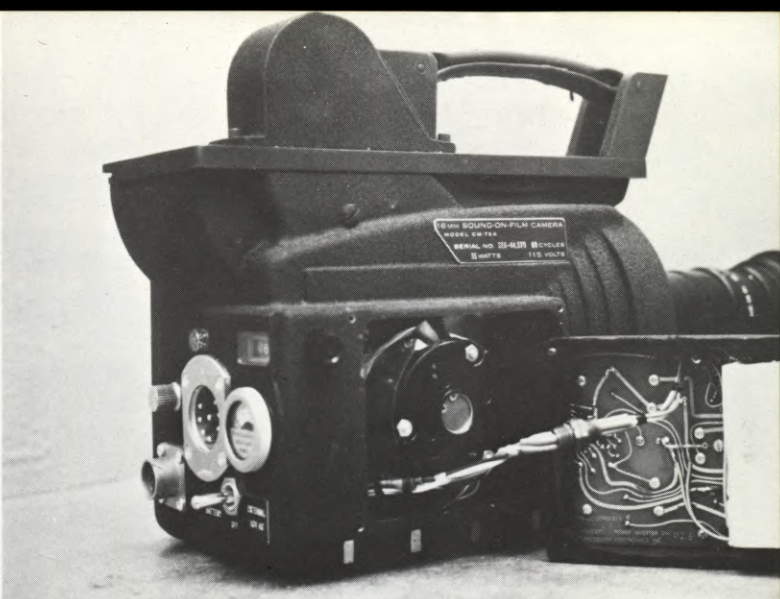
(LEFT) FIGURE 3—Battery installation is both quick and simple. The door is removed and the battery inserted into the connector assembly. Correct polarity will always be observed, due to mechanical polarization of the battery cannister. (RIGHT) FIGURE 4—Left side view, showing easy accessibility of inverter module. The entire electronic circuitry is located within the cover to facilitate servicing. A simple disconnect makes possible quick check-out for periodic maintenance.
