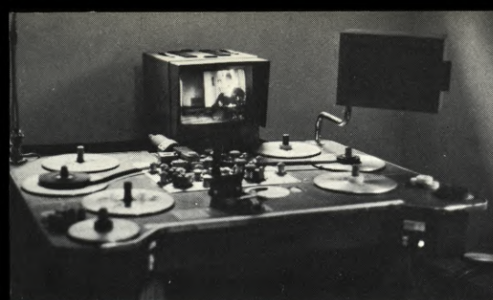
(LEFT) Closed-circuit video monitor linked to Steenbeck editing console at editorial service facility of Dani Shick and Co. Ltd. makes possible reverse-polarity positive viewing of television film negative, plus interlock viewing of picture with two balanced tracks. (CENTER) On the sound stage of Israel Motion Picture Studios, a group of attractive teenagers from the Israeli Army tape a musical show for television. (RIGHT) Young sound mixer is typical of the new generation of technicians now engaged in Israel's film industry.
