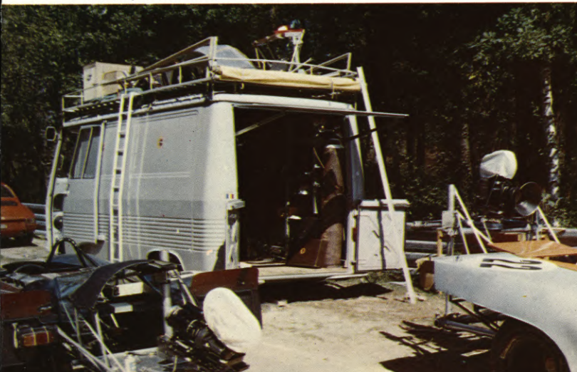
(LEFT) Location van used by camera mount specialist Gaylin Schultz to construct mounts and other special equipment right on the spot. The van accommodates a complete miniature machine shop which Schultz used to build a vast variety of different mounts, dreamed up on the spur of the moment by the director and cameraman. (RIGHT) Schultz (wearing sunglasses) listens to debate about proposed camera mount. When the argument is over, he will make it—whatever it is.
