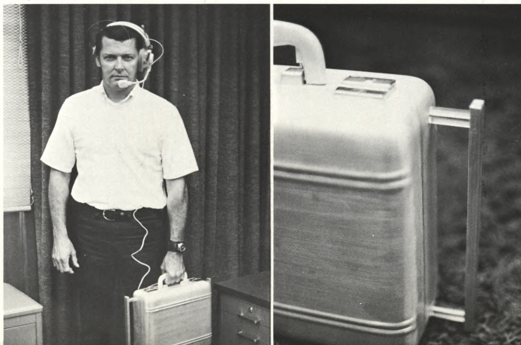
(LEFT) Electronics Engineer Harry Flagle, shown with latest model of wireless intercom transmitter-receiver unit contained in handsome aluminum case. (RIGHT) Sturdy antennas, which look like handles, extend from either side of case. Entire unit will eventually be incorporated into a cordless headset.
