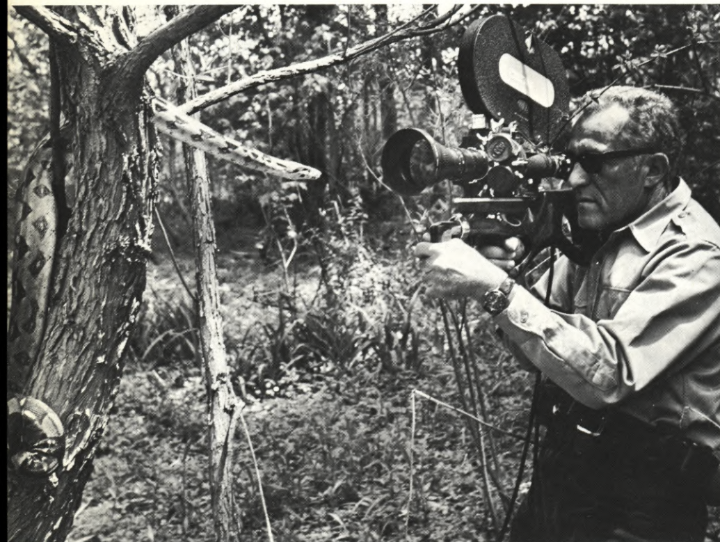
A snake won't wait until you set up your tripod to frame a nicely composed shot of him, and neither will most of the other wild creatures encountered during expeditionary or hunting trips. A gun stock mount assures quick-trigger shooting of a steady picture.
