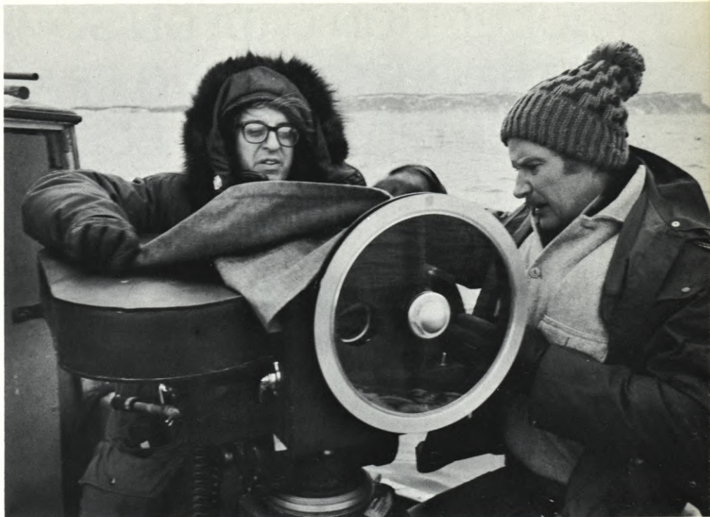
Graeme Ferguson and Assistant Cameraman Ronald Lautore shooting from fishing boat, with camera covered by neoprene barney and circular glass window revolving at high speed to protect lens from spray. This device, regularly used in the wheelhouses of fishing boats during foul weather, was suggested for use in filming by Robert Gaffney, who first utilized it for this purpose in shooting EXPO '70 featurette, "SKY OVER HOLLAND". Rapidly whirling disc not only spins off water drops instantly, but wet snow, as well. A snowball thrown at the disc will be immediately disposed of.
