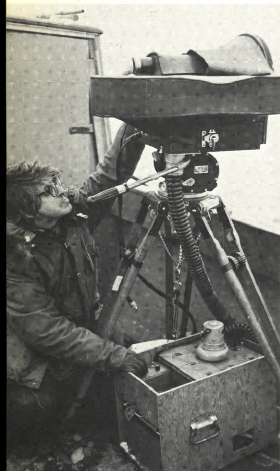
IMAX camera shown completely covered by neoprene "barney" to protect it from extreme cold. Ferguson adjusts portable heater-blower which pumps warm air into covering.
