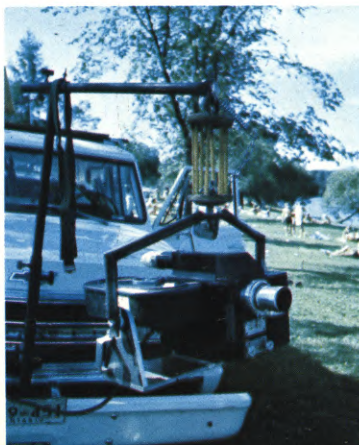
(LEFT) Soundman Avery walks into forest fire area with his recording equipment, accompanied by fire fighter with still camera at the ready. (CENTER) IMAX camera suspended from camera truck bracket by means of F.E.R.C.O. anti-vibration system, which permitted limited "hand-holding" of heavy camera. Developed for use in small helicopter, mount consists of a delicately balanced arrangement of rubber surgical tubing supports. (RIGHT) Most of the shooting of forest fire was done from the top of the station wagon, so that quick escapes could be effected when fire got too close for comfort.
