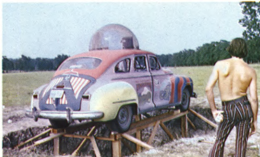
(LEFT) Breakaway platform is built over hole measuring 10' x 20' x 10½' in preparation for sequence to show car being blown up. Fourteen sticks of dynamite and 100 feet of primer cord were placed on the structure. (CENTER) Psychedelically painted car is driven onto platform. Placed in hole were 80 sticks of dynamite, 50 gallons of gasoline and 20 gallons of napalm, with nearly 1000 feet of primer cord laid out in large semi-circle. (RIGHT) Resultant explosion is biggest bang since Hiroshima.
