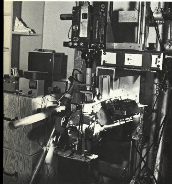
Microscope rig ready to shoot. Sony TV camera views through beam-splitter head. 1000-watt quartz light 10 inches from subject. Pulse motors drive camera, focus, zoom, F-stop, yaw, pitch and roll motions.
