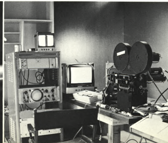
(LEFT) Shooting ultra-closeup of a microtome slicer with F/22 borescope lens made specially for the film by Lenox Instruments. (CENTER) Copy rig used for shooting 35mm film on high-resolution TV monitor. Video processor is behind chair. (RIGHT) Special borescope lens photographing Sorval microtome slicer operated 1/2-inch from subject and covered 60-degree-wide field of view with fantastic depth-of-field.
