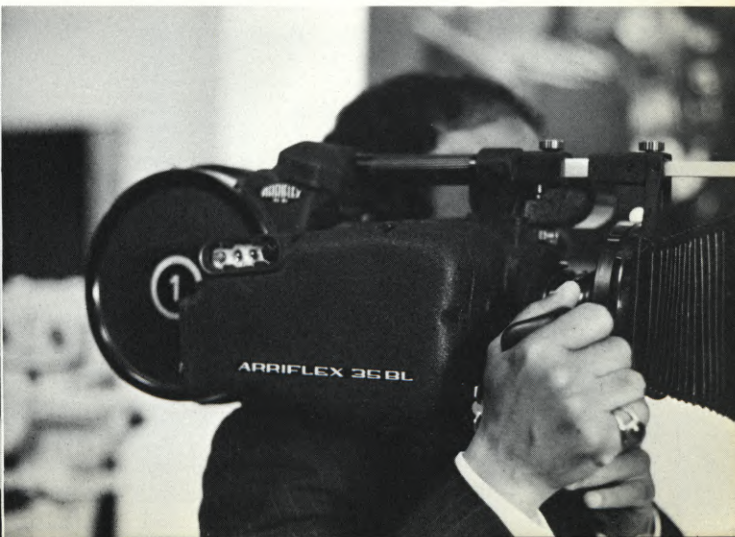
(LEFT) Cinemobile Systems President (and former "I SPY" foreign location Director of Photography) Fouad Said, tries the new Arri 35 BL on for size at Photokina . (RIGHT) The camera's compact configuration and weight-centered coaxial magazine enable it to balance comfortably and securely on the shoulder with no need for a body-brace. Carrying handle on top, designed to serve simultaneously as a matte box rod-holder, makes the camera readily transportable.
