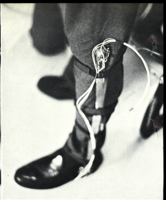
(LEFT) Jones volunteers to have electronic sensors attached to his body so that his movements can be faithfully duplicated by the animated character created within the computer. (CENTER) Detail of the sensor attached to his back and trunk section. (RIGHT) Detail of the sensor attached to his lower leg. Sensors are very light in weight, permitting completely free action.
