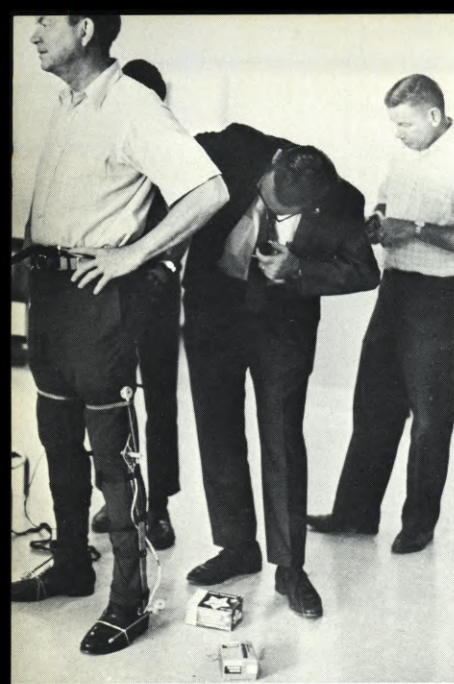
(LEFT) Jones volunteers to have electronic sensors attached to his body so that his movements can be faithfully duplicated by the animated character created within the computer. (CENTER) Detail of the sensor attached to his back and trunk section. (RIGHT) Detail of the sensor attached to his lower leg. Sensors are very light in weight, permitting completely free action.
