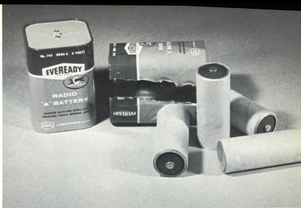
A relatively hard-to-find battery like this 6-volt specimen, when disassembled, is found to be made up of four cells very similar to flashlight cells, except for their length. If taken apart very carefully, the top can be salvaged for use as a connector.
