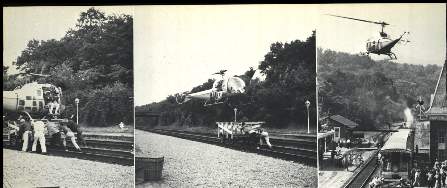
Photo series showing the progression of a helicopter shot made by Nelson Tyler, using the vibrationless camera mount which he designed. (LEFT) Helicopter on flat car is pushed along the railroad tracks by grips to achieve a "soft" start. (CENTER) The craft lifts off of the flat car, continuing the backward motion as it rises. (RIGHT) The helicopter soars above the train as it moves out of the station, and follows its journey along the riverbank.
