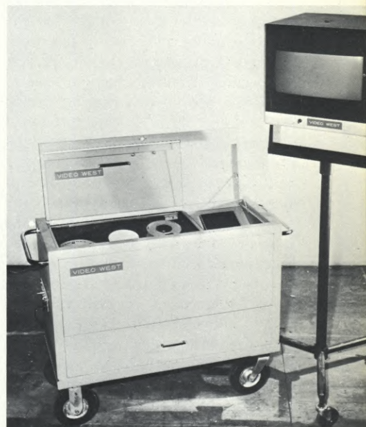
(LEFT) Console of the Video West system serves as control center and contains an Ampex 660 2-inch helical-scan video tape recorder and a small monitor. (RIGHT) Floor monitor for use on the set.
