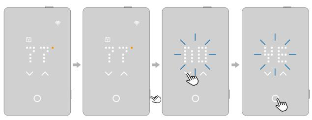
In the screen saver mode, touch the **temperature** area to wake up the thermostat. The home screen will appear.
