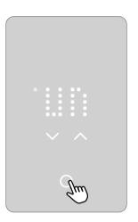
Press the **select/accept button** to confirm the setting.
