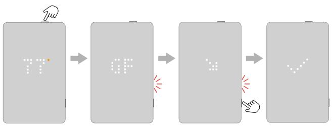
Press the **top button** to test the GFCI relay.
