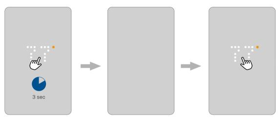
In the screen saver mode, press the **temperature** area for three seconds and the screen will turn off.
