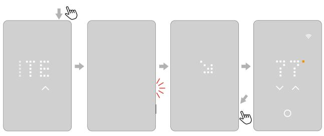
Push the **top button** to test the GFCI relay.
