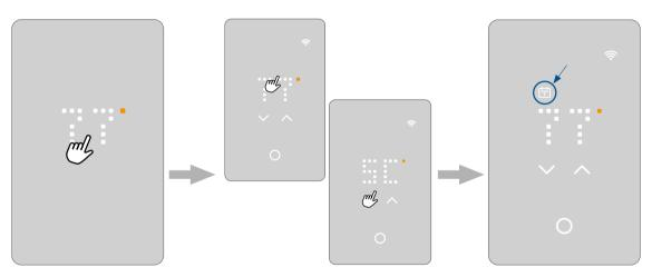
In the screen saver mode, touch the **temperature** area to wake up the thermostat. The home screen will appear.
