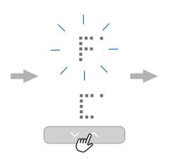
Press the up or down arrow to set the temperature unit to Fahrenheit or Celsius.
