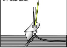
Step 18: Make connections. Connect the power wires to the cable wires, and the ground wire to the cable braid. Wire nuts (D) cannot be connected with aluminum wires. Ground the junction box. For heating cables with outer jacket, see shown figure.
