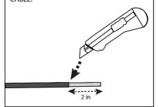
Step 2: Push back the braid to expose the cable. Cut off the end 3/4" of the cable. To prevent short circuits, do not connect bus wires. Keep braid away from shrink cap. WARNING: ELECTRIC SHOCK HAZARD
