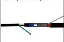
Step 19: Slide and center the tube closest to the splice (B) (5") over splice, making sure it extends over the end of cord and cable.
