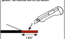
Step 6: Bend to break where scored and peel off outer jacket.
