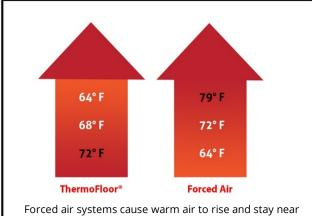
Forced air systems cause warm air to rise and stay near the ceiling. ThermoFloor®'s radiant floor-to-body heat starts and stays with you, feeling 6-8 degrees warmer and saving up to 40% energy.
