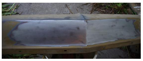
The Dodge letters on the front header had been removed before I got the car. I filled the holes with the MIG, same for all the holes down the side of the car where the trim was.
