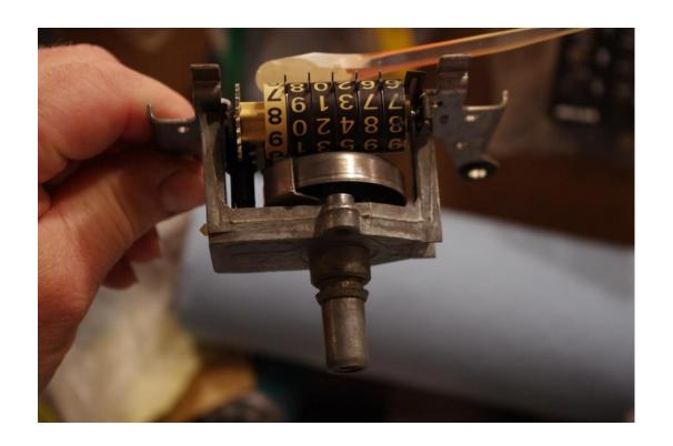
When I started driving the speedometer needle would sometimes start bouncing. I took it in and out of the dash a bunch of times. I was hoping for it to be the cable, but it was not. I started to bench test it with a drill but couldn't solve the problem. It appears the bushings are worn and the spinning magnet occasionally drags on the needle bar. Hard to find mechanical speedo rebuilders!
