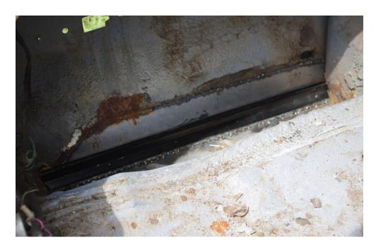
The inner trunk pan needed a couple of inches of new metal and then I put this right angle piece in for the cards that slide in to protect the quarter panel. The piece was already painted black as I cut it out of a repop rocker panel for a Buick Park Avenue that was laying around.
