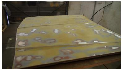
Both the hood and roof had some surface rust popping through, I spot blasted / ground them and feathered out the spots.
