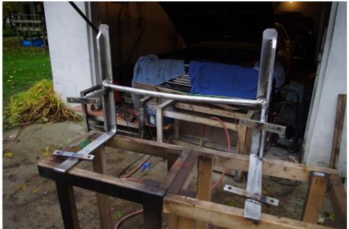
After painting the car I started work on the push bar. Lused the liquidrealities plans. Thanks to them for sharing! I'm glad I got them when I did as I think they are down now. My local steel shop could not put the 1 inch cross bar in their roller for the bend. I made up a jig and put a lot of heat into the bar to get it bent. When complete this is one hefty piece. I elected not to weld it on the frame, I just went with the bumper mount.
