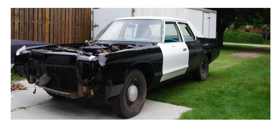
By the end of August 2018 it was looking more like a car. I used Sherwin-Williams Automotive Industrial Coatings acrylic enamel single step paint. The 1975 Body Service manual says the paint used was acrylic enamel so I guess I am period correct. I used the hot weather reducer and a splash of hardener. It still took a week to dry hard. The cold weather was coming so the graphics waited till next year.
