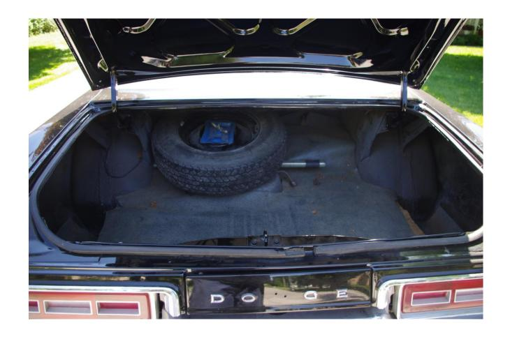
The car came with the trunk mat and jack with handle. I saw in the sales folder that a Police option was a single key for all locks. I pulled some pins out of the trunk tumbler to make that happen. I now have one police option on the car and it was a whole lot easier than some of the others on the list!
